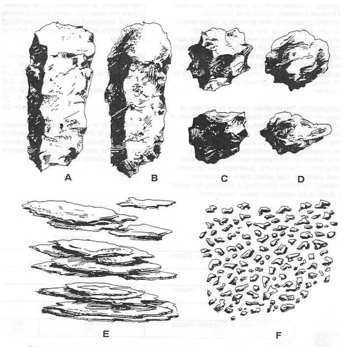
Drawings illustrating some of the types of soil structure: A - prismatic; B - columnar; C - angular blocky; D - subangular blocky; E - platy; and F - granular <u>Excessively drained</u>. Water is removed from the soil very rapidly. Excessively drained soils are commonly very coarse-textured, rocky, or shallow. Some are steep. All are free of mottling related to wetness.
